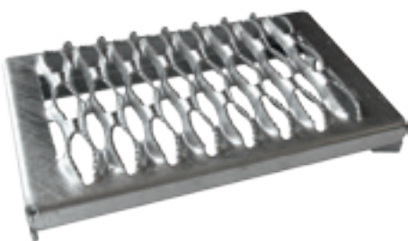
Tread of type Graepel-Stabil, hot-dip galvanized steel, all-round welded-on with integrated stepping edge
